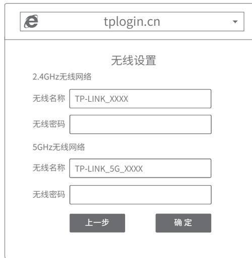
The screenshot shows the '无线设置' (Wireless Settings) page. It is divided into two sections: '2.4GHz无线网络' and '5GHz无线网络'. Each section has input fields for '无线名称' (Wireless Name) and '无线密码' (Wireless Password). The 2.4GHz name is 'TP-LINK\_XXXX' and the 5GHz name is 'TP-LINK\_5G\_XXXX'. At the bottom are two dark grey buttons: '上一步' (Previous Step) and '确定' (Confirm).
